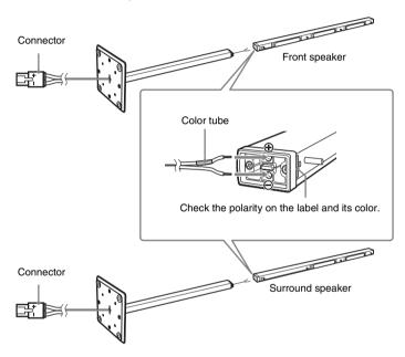
Insert the speaker cords into the speaker terminal of the speaker as far as they will go. Ensure that the cords are secure by gently pulling on them one at a time.
